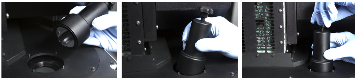
Figure 4.19 Inserting the Filter Tool Into the Filter Wheel Access Opening
